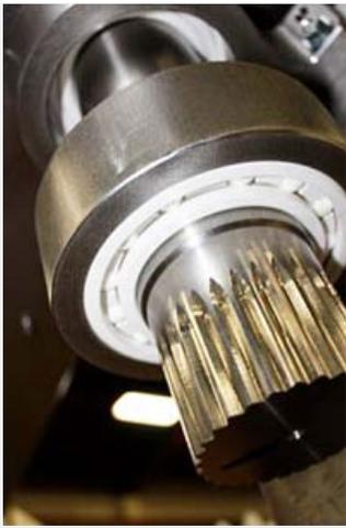
The clock uses a number of materials, including titanium and ceramic, seen here in white. (Courtesy of Long Now)
